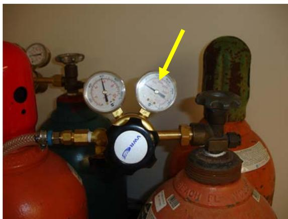
**Figure 1:** Read the N<sub>2</sub> cylinder pressure (dial indicated by yellow arrow) and record in logbook at start and end of glovebox use.
