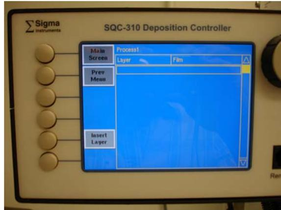
**Figure 15:** Connect your film to the process by pressing *Insert Layer*.
