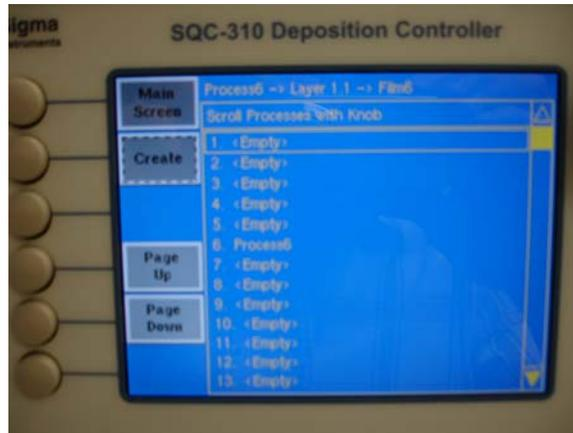
**Figure 13: Creating a process on the SQC-310 deposition controller.**
