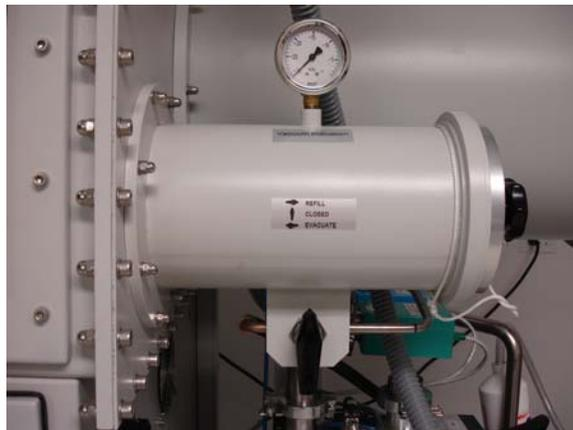
Figure 4: Mini-antechamber under static vacuum.
